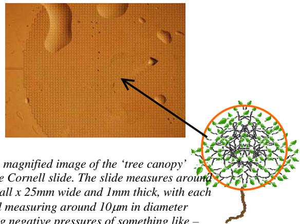
*A much magnified image of the ‘tree canopy’ from the Cornell slide. The slide measures around 60mm tall x 25mm wide and 1mm thick, with each channel measuring around 10µm in diameter inducing negative pressures of something like – 1.0MPa*
