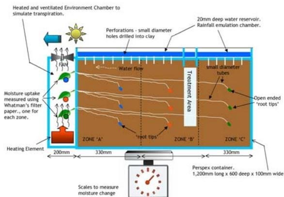
*Diagrammatic view of the model showing (left) the 'environment chamber', enclosing the heater and fan, controlling relative humidity and right, the chamber containing the soil, treatment zone and 'roots'. The model includes a rainfall chamber situated above the soil. Tubes (roots) pass between the chambers to establish a flow driven by relative humidity.*
