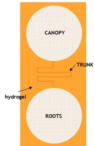
This is the rationale behind building our own ‘synthetic tree’. As the environmental factors can be controlled it will form the basis of a mathematical model allowing us to understand better the complex interaction between rainfall, temperature, hydraulic conductivity and root absorption without having to worry about carbon fixing, hours of sunshine, stomatal response and photosynthesis.
